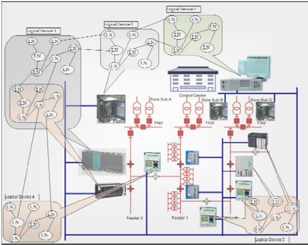
Figure 3. Proposed approach: distributing the control and functions to the autonomous intelligent component.
